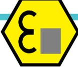
Marking of equipment where an explosive atmosphere can be formed.
